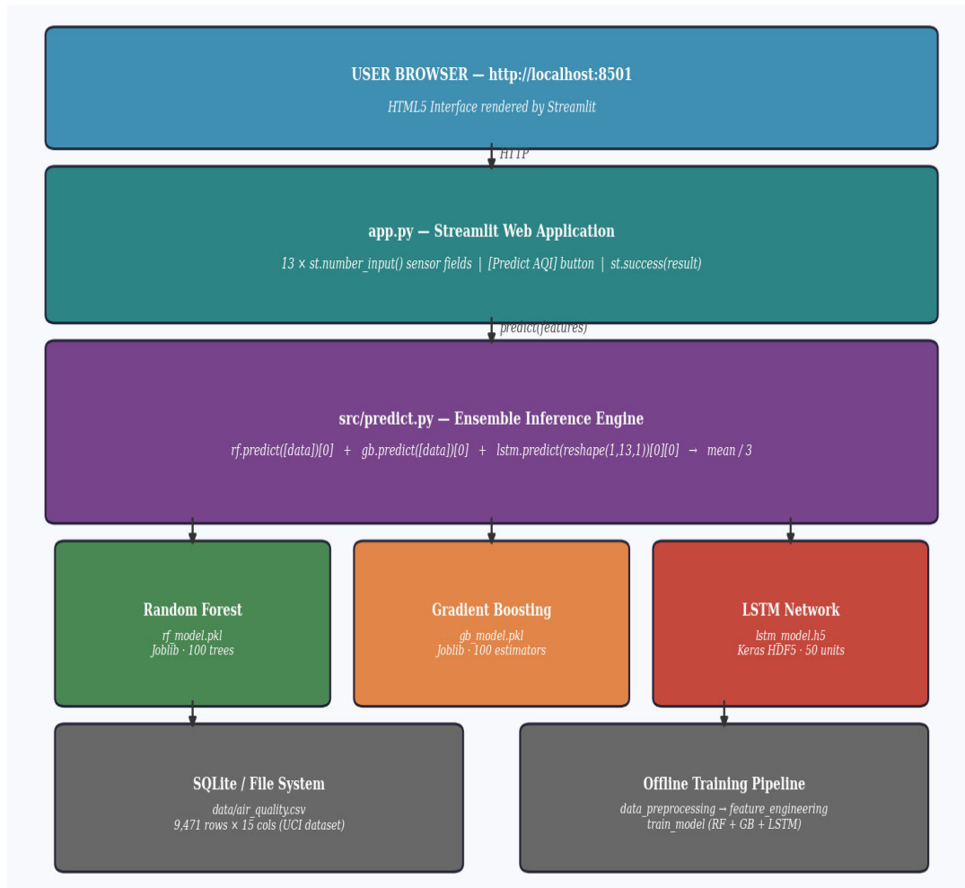
Figure 1: AirGuardPlus AI three-tier system architecture showing the Streamlit Presentation Tier, the Ensemble Inference Engine with three model artifacts, and the Offline Training Pipeline processing the UCI Air Quality dataset.
